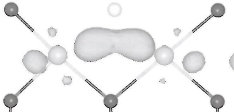
Figure 1. The density of electrons at the oxygen vacancy at TiO 2 (110) (indicated with fictitious white sphere).
